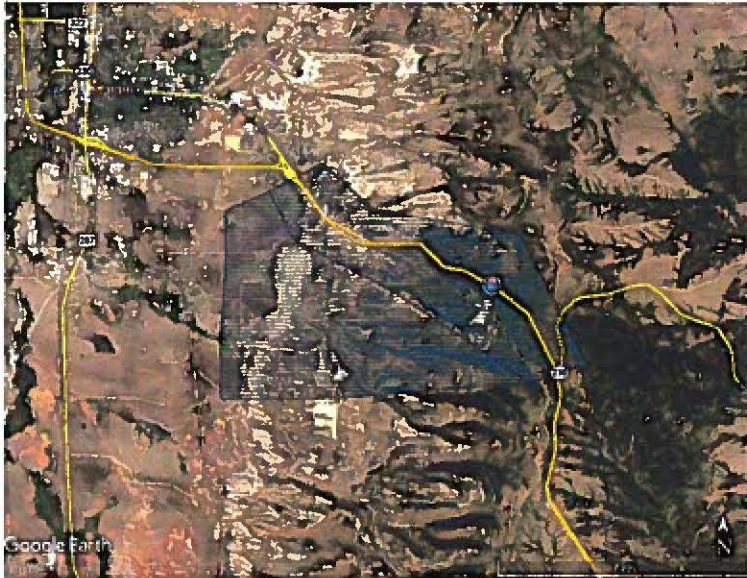
Figure 1. 2019 I-80 Airborne Electromagnetic Survey area. Blue lines are the flight tracklines for the helicopter survey. The I-80 WyDOT right of way is not covered due to FAA regulations. However, both sides of I-80 immediately outside of the interstate right of way will be covered. Tracklines are shown at 100 m (~330 ft.) intervals over the survey area. This is a preliminary map of the survey area for budget estimation purposes. The final flight transects will be modified to avoid/minimize any overflight of residential areas and infrastructure (e.g. powerlines).
